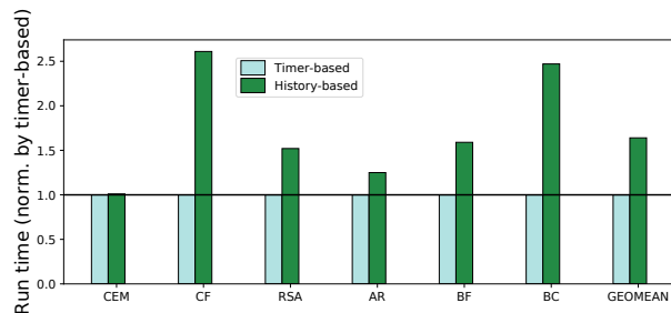
Figure 12: Run time of two different heuristics. Run time of timer-based checkpoint disabling versus history-based checkpoint disabling.
